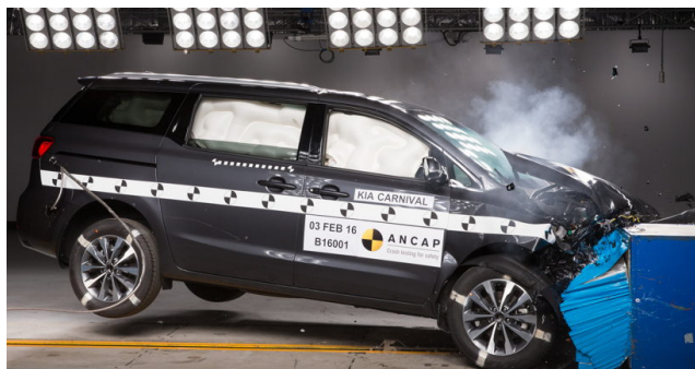
Frontal offset test at 64km/h
