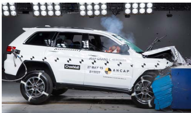
Frontal offset test at 64km/h
