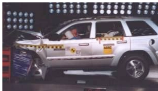
Offset crash test at 64km/h
