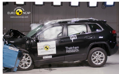
Frontal offset test at 64 km/h (Euro NCAP)
