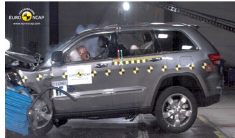
Offset crash test at 64km/h
