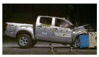
Frontal offset test at 64 km/h (D-Max utility tested by ANCAP)
