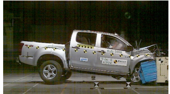
Frontal offset test at 64 km/h (D-Max utility tested by ANCAP)
