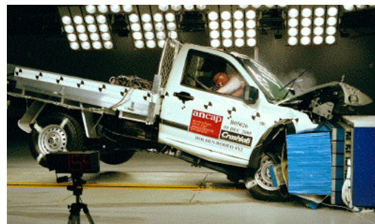
Offset crash test at 64km/h
