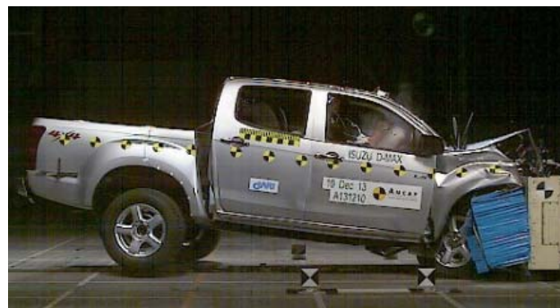
Frontal offset test at 64 km/h
