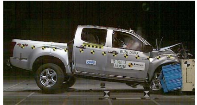
Frontal offset test at 64 km/h
