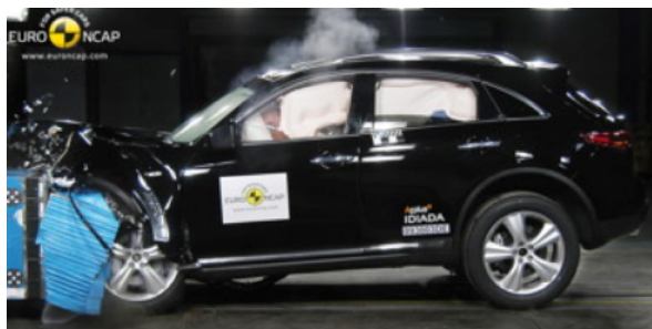
Offset crash test at 64km/h (Euro NCAP)
