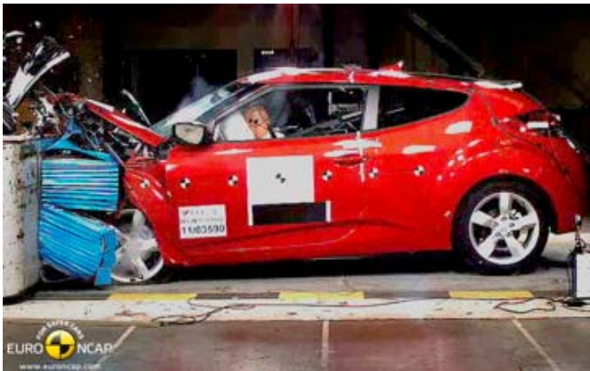
Frontal offset test at 64km/h
