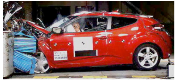
Offset crash test at 64km/h (Euro NCAP)
