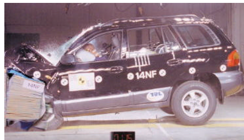
Offset crash test at 64km/h
