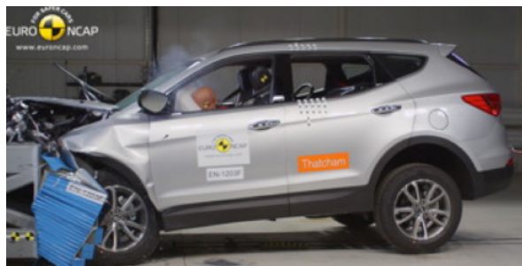
Offset crash test at 64km/h (Euro NCAP)
