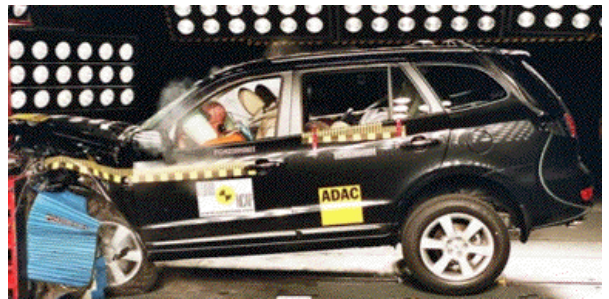
Offset crash test at 64km/h
