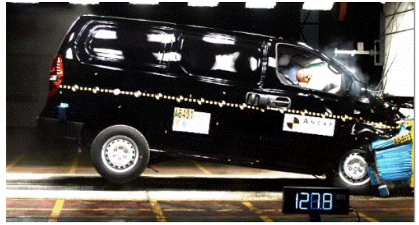
Offset crash test at 64km/h (iLoad van)
