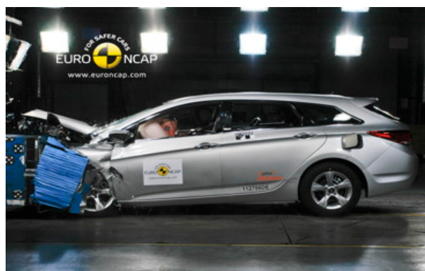
Frontal offset test at 64km/h
