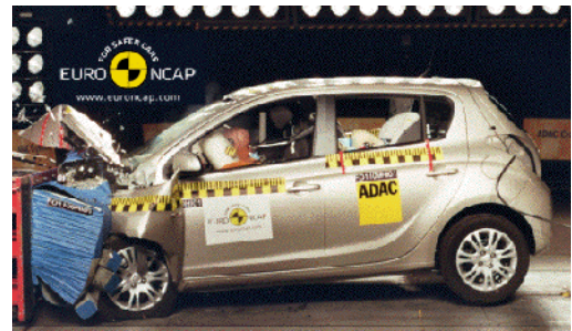
Offset crash test at 64km/h
