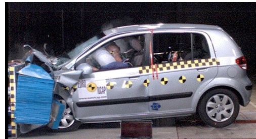
Offset crash test at 64km/h
