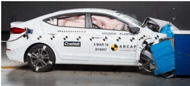
Frontal offset test at 64km/h
