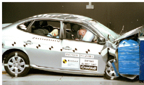
Offset crash test at 64km/h
