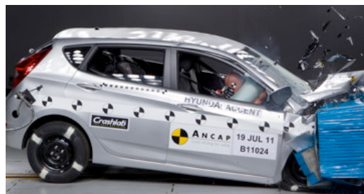
Offset crash test at 64km/h
