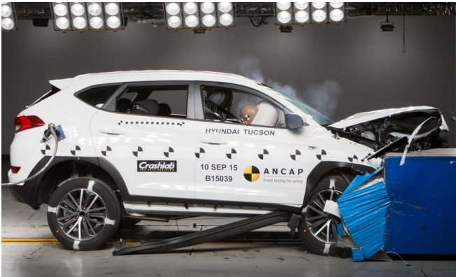
Frontal offset test at 64km/h
