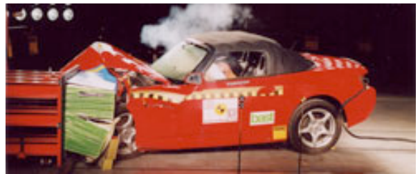
Offset crash test at 64km/h
