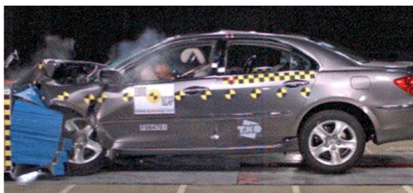
Offset crash test at 64km/h
