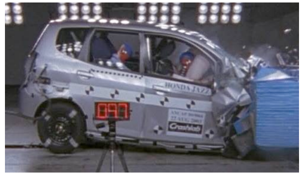
Offset crash test at 64km/h
