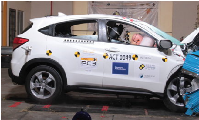
Frontal offset test at 64km/h (ASEAN NCAP)
