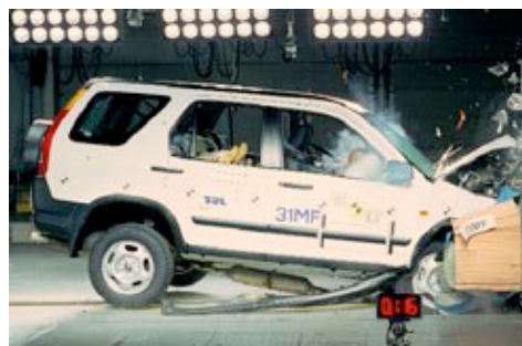
Offset crash test at 64km/h
