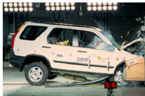
Offset crash test at 64km/h
