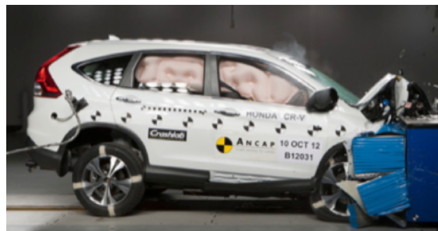
Frontal offset test at 64 km/h
