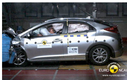
Offset crash test at 64km/h
