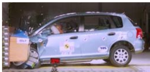
Offset crash test at 64km/h
