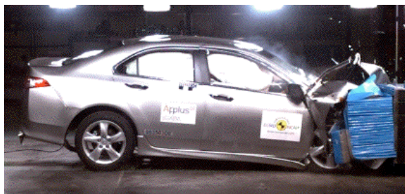
Offset crash test at 64km/h
