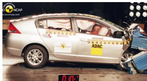
Offset crash test at 64km/h
