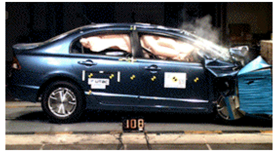
Offset crash test at 64km/h
