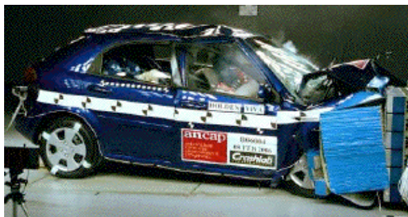
Offset crash test at 64km/h
