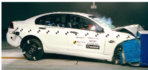
Offset crash test at 64km/h (Commodore)
