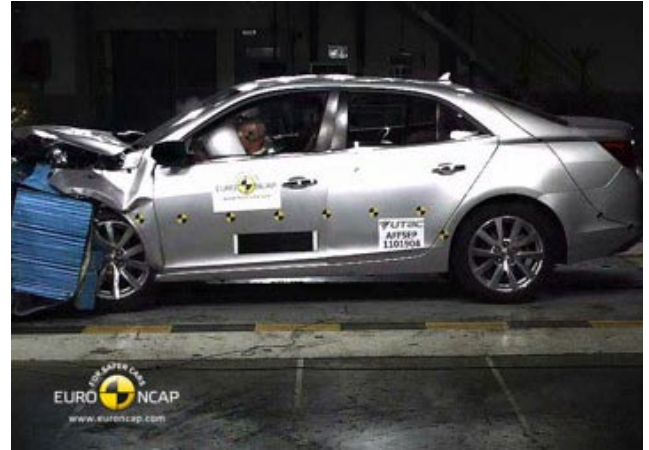
Frontal offset test at 64 km/h (Euro NCAP)
