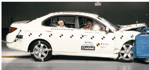
Offset crash test at 64km/h
