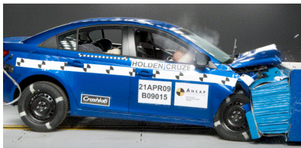
Offset crash test at 64km/h
