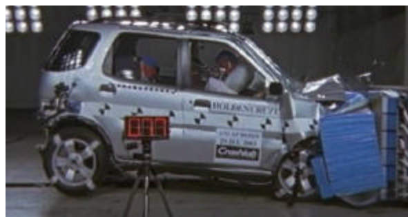
Offset crash test at 64km/h
