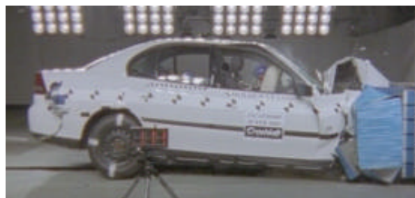
Offset crash test at 64km/h
