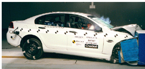
Offset crash test at 64km/h
