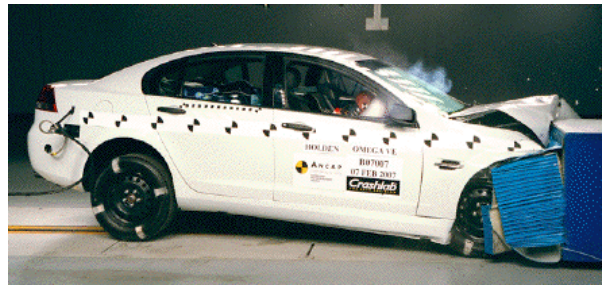
Offset crash test at 64km/h
