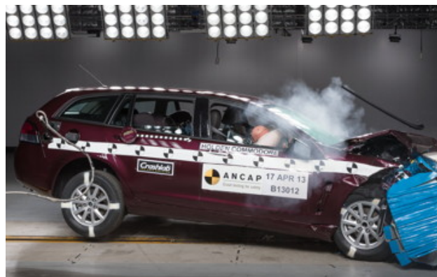
Frontal offset test at 64 km/h (Commodore wagon)
