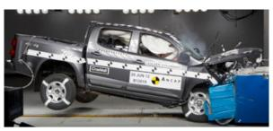
Offset crash test at 64km/h (Colorado Utility)
