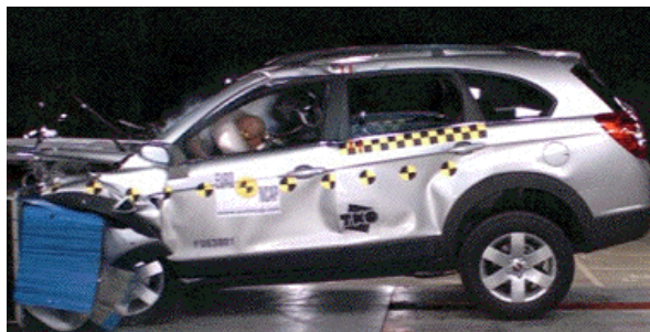
Offset crash test at 64km/h
