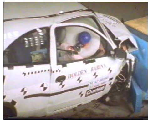
Offset crash test at 64km/h
