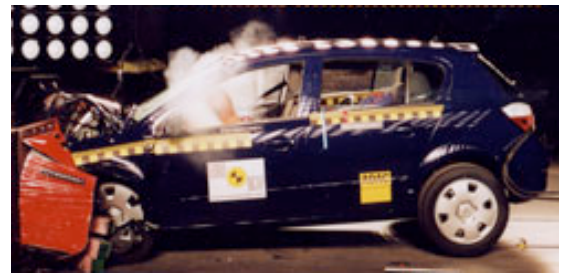
Offset crash test at 64km/h
